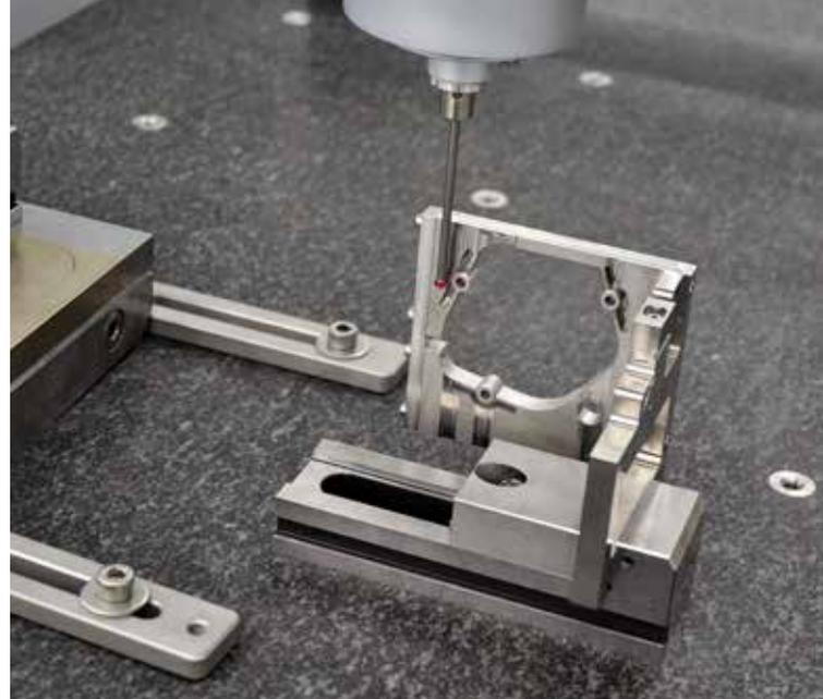
*High-precision measurement of a component for a lithography system.*
