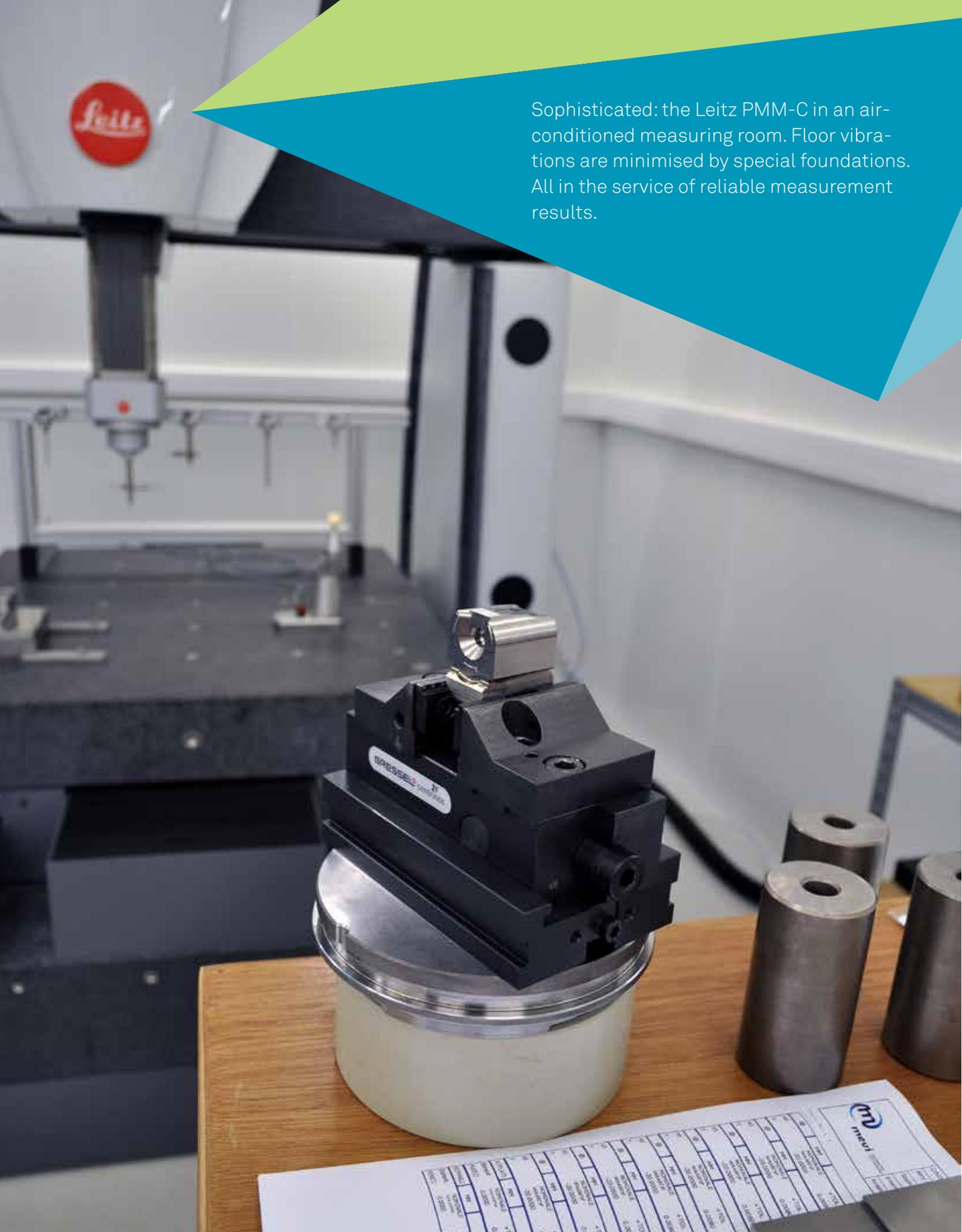
Sophisticated: the Leitz PMM-C in an air-conditioned measuring room. Floor vibrations are minimised by special foundations. All in the service of reliable measurement results.
